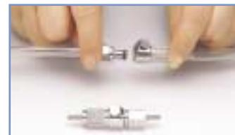
in-line connections and automatic shut off when disconnected. Hose barb ends accept flexible tubing. Operate at temperatures to 82°C (180°F), pressures to 1.7 Mpa (250 psi), vacuum to 30 microns of Hg. Chrome plated valves provide dependable operation; ideal for liquid and gas connectors in biomedical instrumentation and general industrial applications.
